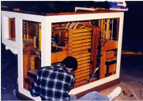
The console before restoration. Stan is beginning to remove the old pneumatic action. Note that the console was painted.
