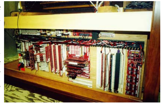
The "main brain" of the Peterson system located in the console
