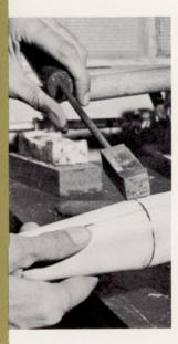
Soldering the foot and body sections of a metal pipe.
