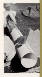
Soldering the seam of a reed pipe resonator.
