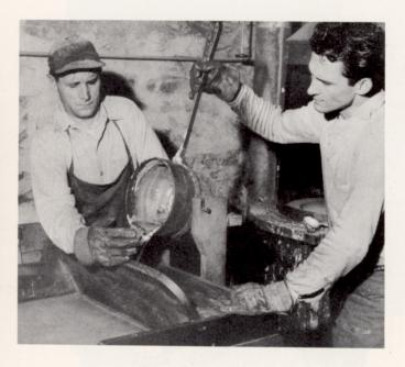
Pouring of the molten tin and lead which will be formed into a sheet of pipe metal.
