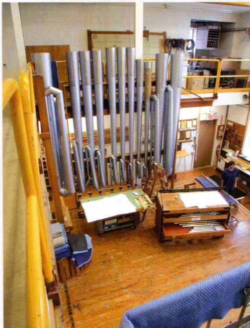
▲ The 13 largest pipes of the 32' Ophicleide being voiced in the assembly room
