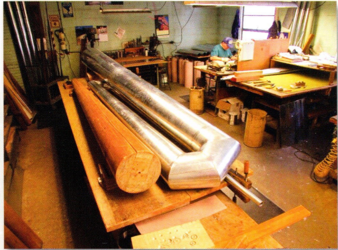
▲ The resonator for low C# of the 32' Ophicleide (pedal reed)
