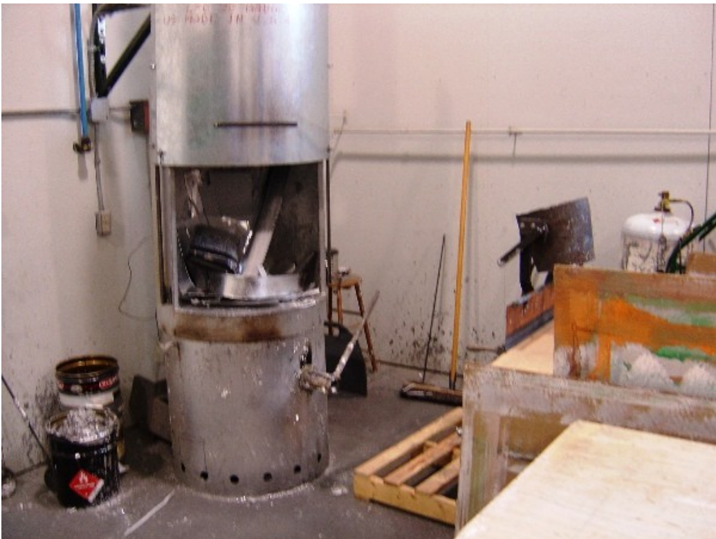
Figure 12: Forge for melting pipe metal
