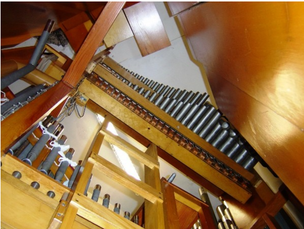
Figure 8: Great upper (Choir) chest and Harp, view looking up the ladder toward the ceiling. Clarinet in foreground lower left; Pedal Open Diapason (wood) on the right.
