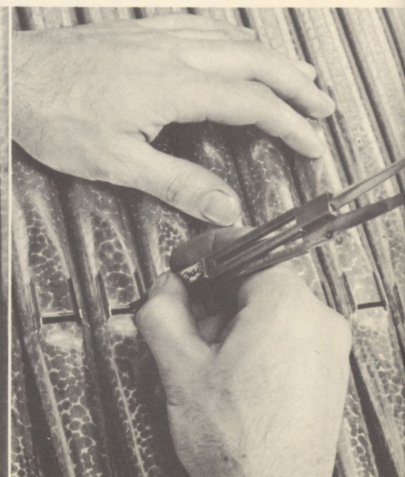
Marking the "cut-up" of the lips of a set of metal pipes
