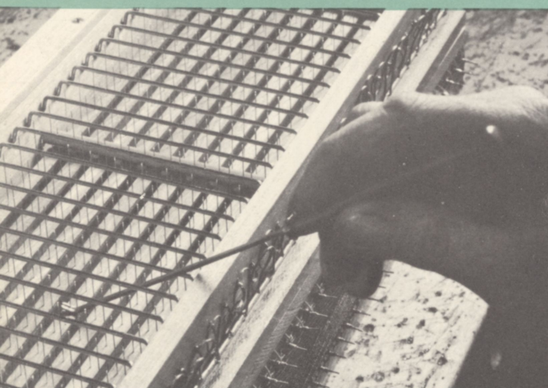
Making final adjustment of contacts in the key action switch
