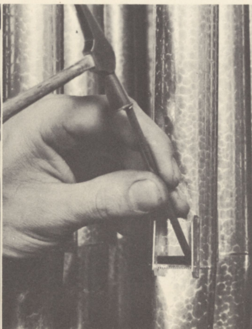
Adjusting the "languid" of a metal pipe
