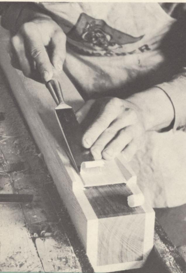
Preliminary cutting of the upper lip of a wood pipe
