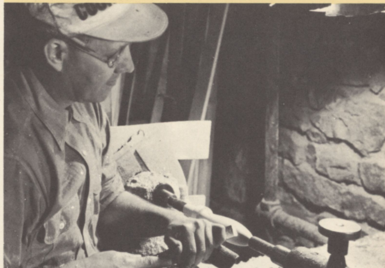
Turning handle for stopper of a wood pipe
