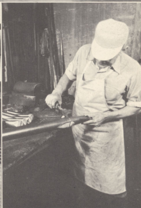
Soldering together the foot and body sections of a metal pipe
