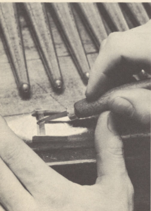
Nicking or "cutting the teeth" in a metal pipe
