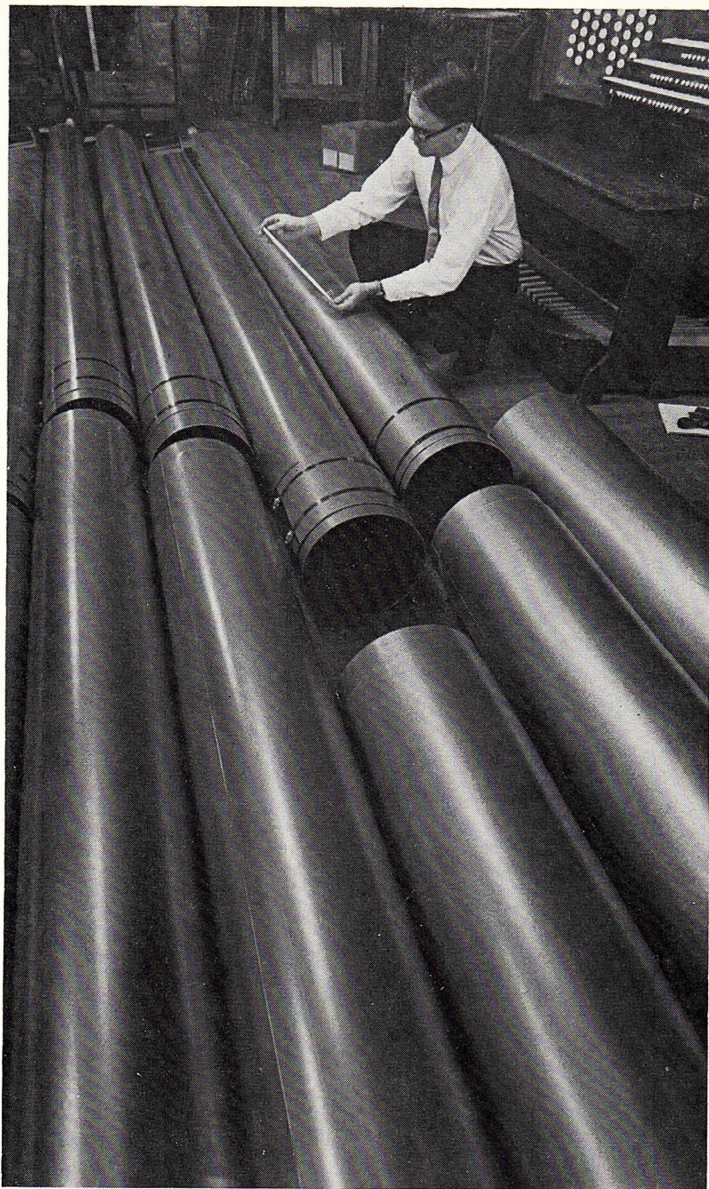
The Kontra-Violon, disassembled at the factory and ready for shipment, compared in size to one of the larger mixture pipes.
