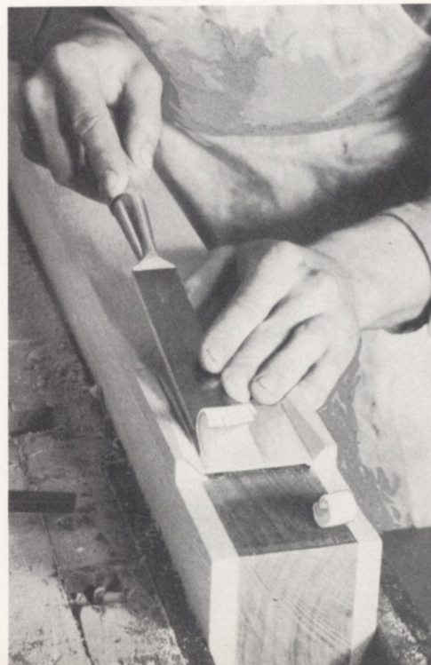
PRELIMINARY CUTTING OF THE UPPER LIP OF A WOOD PIPE
