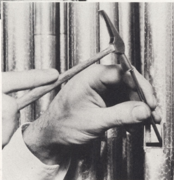
ADJUSTING THE LANGUID OF A METAL PIPE
