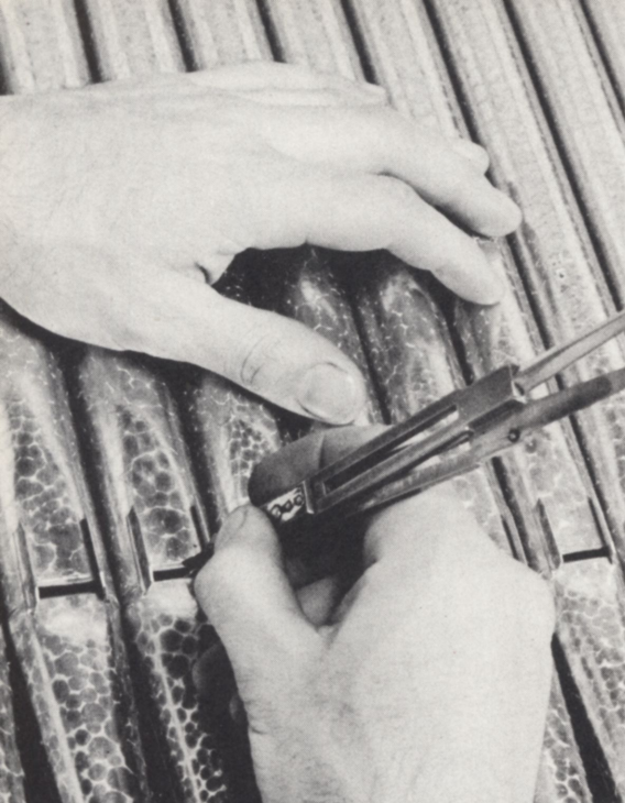
MARKING THE "CUT-UP" OF THE LIPS OF A SET OF METAL PIPES
