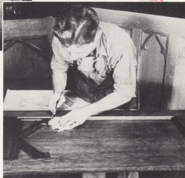
STAINING THE END SECTION OF A CONSOLE CASE
