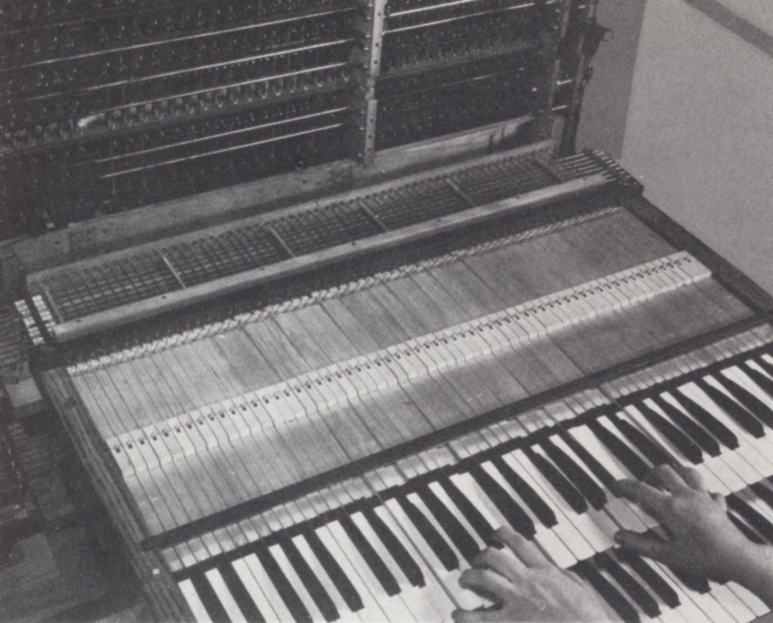
THE REUTER KEY ACTION MECHANISM. THE DEPRESSING OF THE KEY BY THE FINGER LIFTS THE BACK END OF THE KEY WHICH IN TURN MOVES THE ARM OF THE CONTACT ROLLER, CAUSING THE ROLLER TO EXERT A GENTLE RUBBING ACTION AGAINST THE CONTACT WIRE
