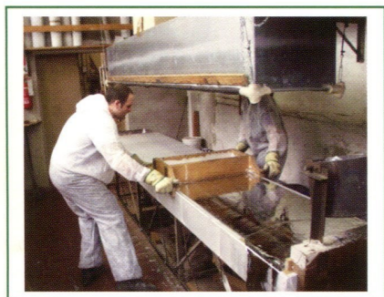
One step in the melting process at the Ruffatti factory used to create the tin and lead alloy for metal pipes.
