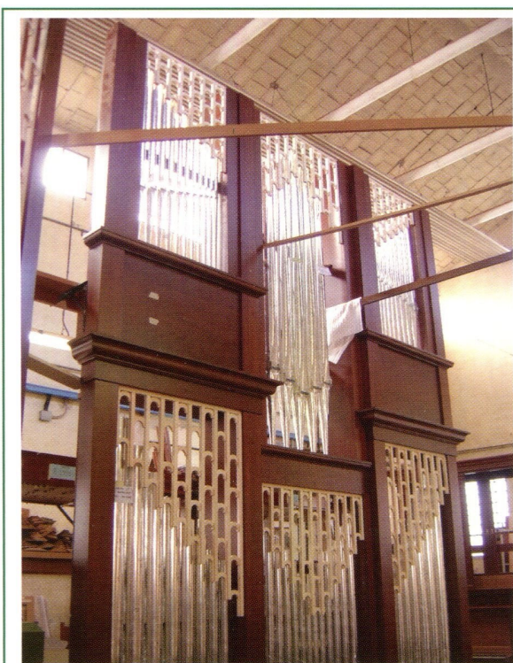
One of the pipe facades for the Johns Creek Baptist Church organ, erected in the Ruffatti factory prior to being disassembled for trans-Atlantic shipping.
