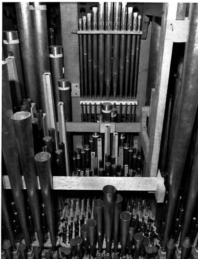
Manual pipework, including lead tubes to façade pipes
