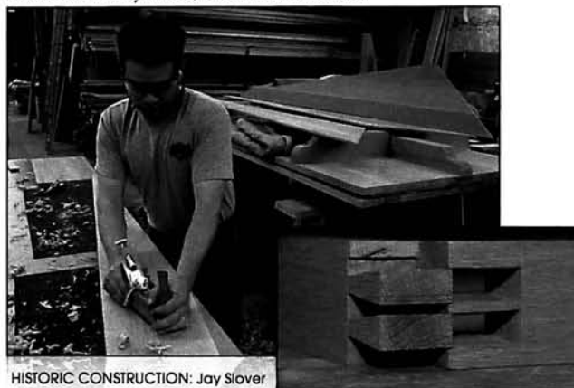
HISTORIC CONSTRUCTION: Jay Slover hand planing quarter-sawn oak (left). Dove tail joints were essential in a historic 18th century organs (right).
