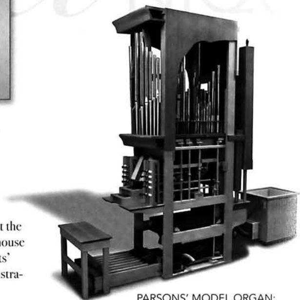
PARSONS' MODEL ORGAN: Educational tool for schools, one octave cross section of a two manual tracker pipe organ
