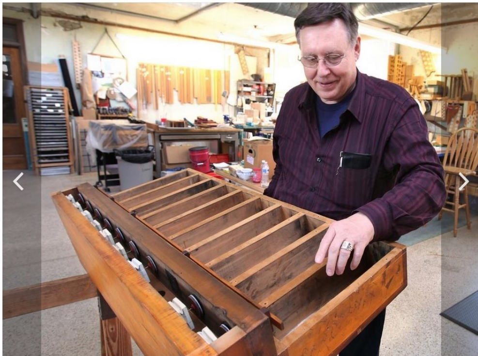
Phil Minnick, co-owner of Bunn-Minnick Pipe Organs, is pictured with an organ stop-action that is having wood splits repaired by his company.
