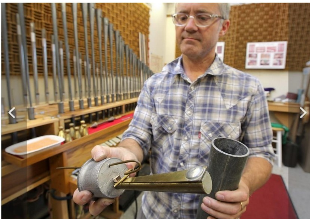
Organ voicer Scott Gorsuch of Bunn-Minnick Pipe Organs in Columbus shows the reed/tongue assembly of an organ owned by Sacred Heart Church of Cincinnati. The organ was originally constructed in 1895 by A.B. Felgemaker of Erie, Pa.
