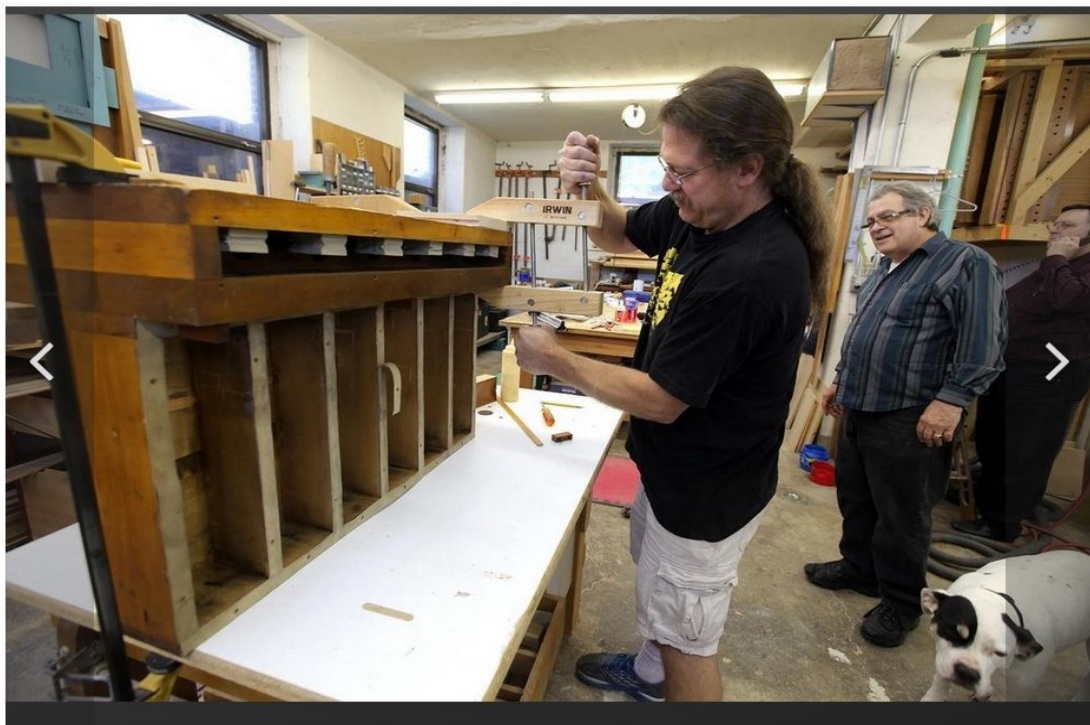
Gary Gould of the Bunn-Minnick Pipe Organ Co. works on restoring wood splits on an organ stop-action piece in the shop. Also pictured are company owners Robert Bunn (center) and Phil Minnick (far right). Shop dog Clover is pictured at bottom right.
