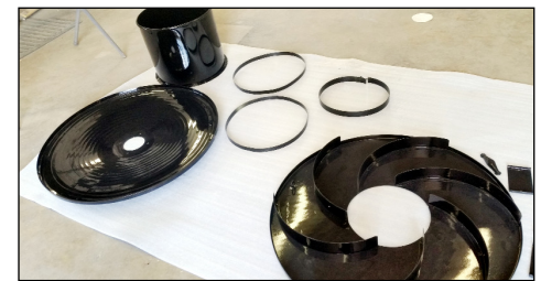
Motor plate, intake tube, bands and finned separator plate
