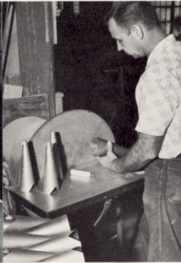
Smoothing the edges of zinc pipe feet prior to soldering.
