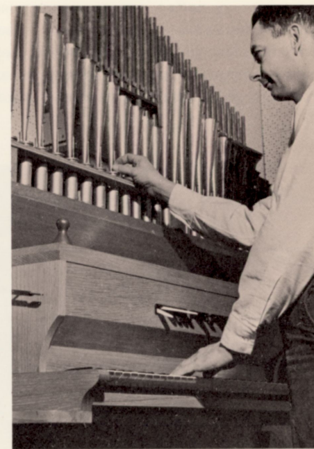
One of the reed pipe voicing rooms. The set of pipes being voiced is a trumpet.
