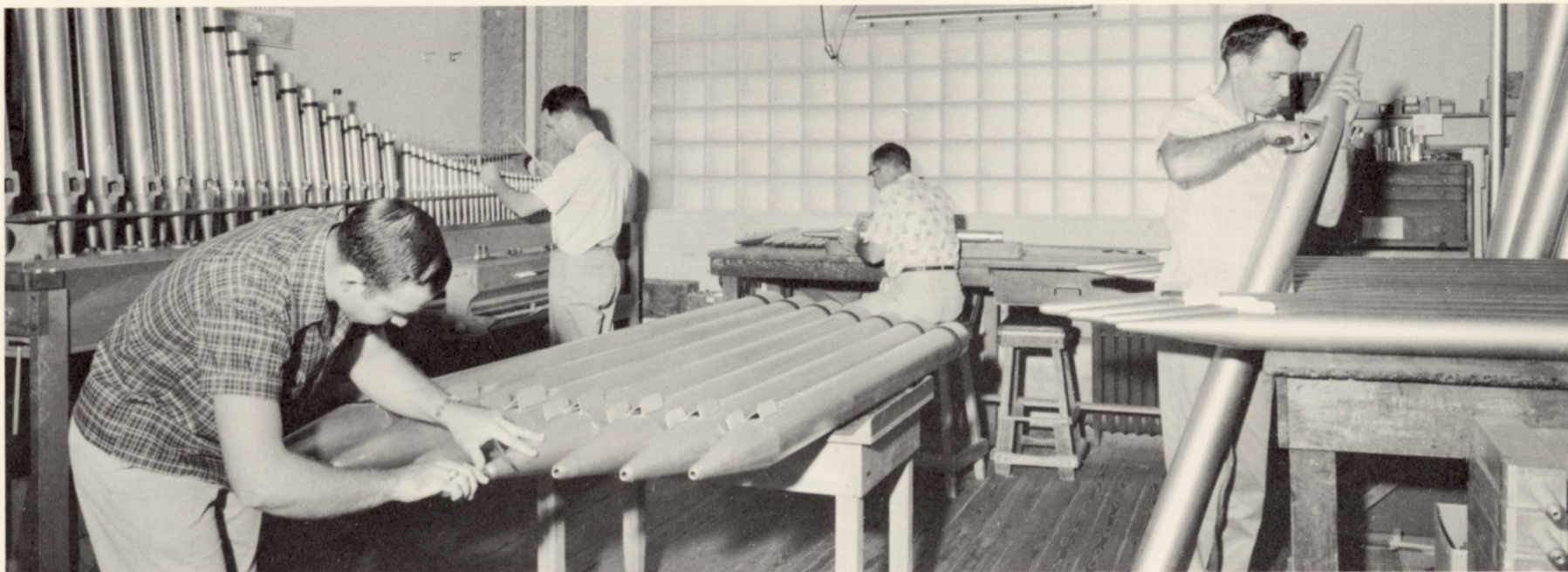
One of the flue voicing rooms. Pipes are shown in the process of preparation and voicing.
