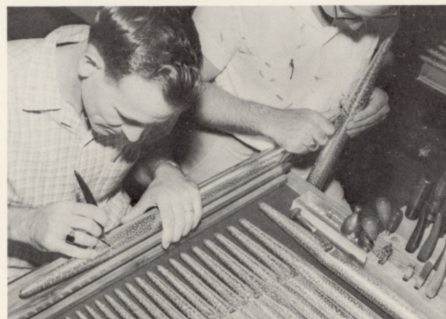
Making the "cut-up" on the upper lip of a metal pipe.
