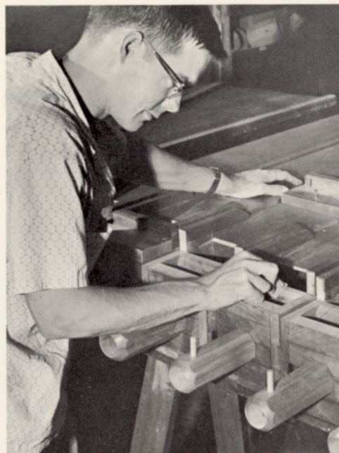
Final sanding of the languids of wood Bourdon pipes.
