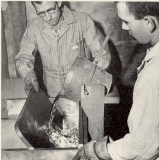
Pouring of the molten tin and lead which will be formed into a sheet of pipe metal.
