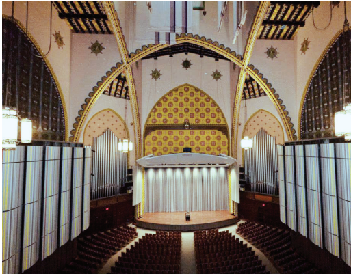
Irvine Auditorium: Interior. A grand space for a grand instrument. The majority of the organ is installed behind the stenciled scrims visible at left and right. A portion only of the Pedal Division is housed behind the non-speaking façade pipes. Grey reflector panels were installed in the 1997-2002 renovations.
