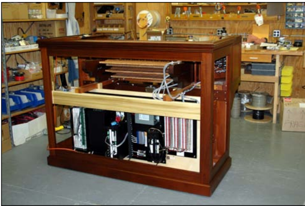
Inside of console showing computer control system.
