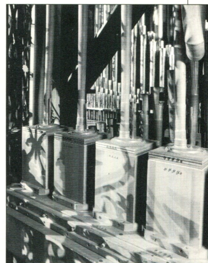
Virgil Fox at the 1948 console (top); Æolian-Skinner added two new 32' registers: the Bombarde (above), and the Contre Gambe (middle), whose feet and mouths are traditionally built but whose bodies are made of flexible hose.
