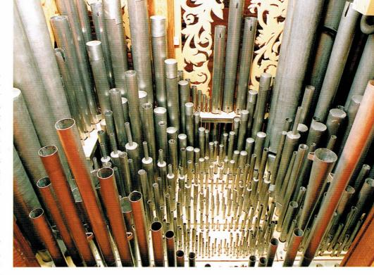
Completing the pipes in the Great are four sets of reed pipes, which work somewhat like clarinets; three belong to the trumpet family and have conical resonators and a very strong tone. The remaining reed is the Hautbois, a set of pipes organ builders created to imitate the precursor of the modern oboe; it is useful for all kinds of solo effects.
